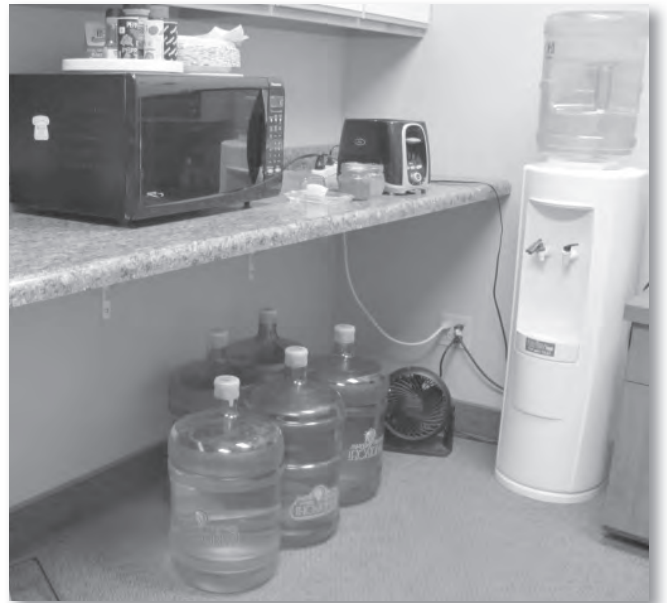
The water jugs are obstructing a person's leg room below the counter. Individuals who utilize a wheelchair may have a difficult time accessing the counter space.
