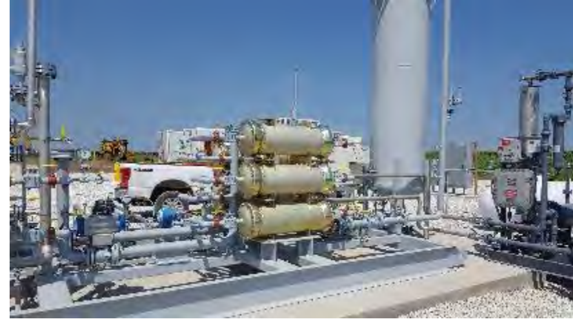
Raw biogas (64% CH 4 , 35% CO 2 ) is cleaned to >96% CH 4
