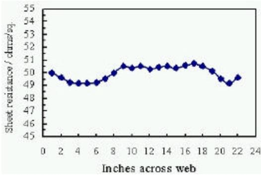
**Figure 1 - Sheet Resistance Across a Resistive Foil Web - NiCr, 50ohm/sq. on 1/2oz Reverse Treated Foil**
