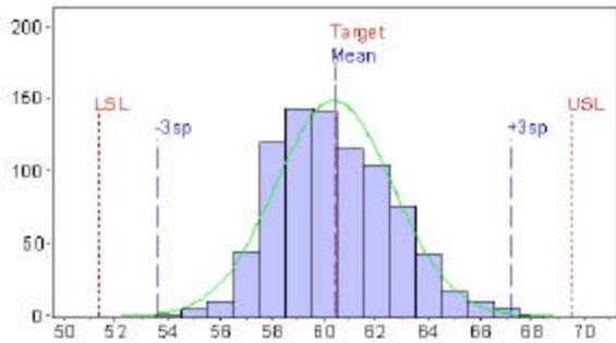
**Figure 9. 20 mil Resistor Data Compared to a Target of 60 ohms - Predicted Yield is Greater than 99%**
