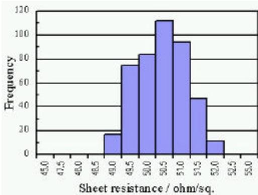
**Figure 2 - Statistic Results of 440 Sheet Resistance Measurements on a 500ft Production Roll - NiCr, 50ohm/sq. on 1/2oz Reverse Treated Foil**
