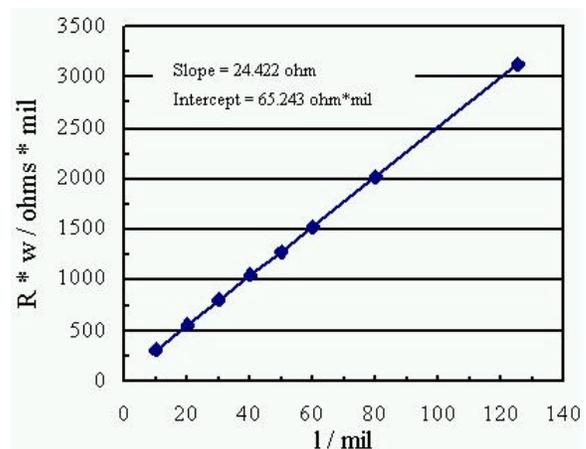
**Figure 5 -  $Rw$  vs.  $l$  Plot to Calculate the Total Amount of Resistor Length Compensation - Data are from Table 2, STD Foil - Calculated Total Amount of Resistor Length Compensation is 2.66mil**
