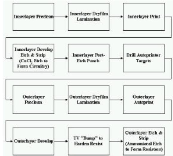
Figure 8 - Flow Diagram Showing Process for Forming Resistors with TCR Material
