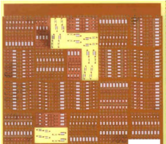
Figure 6 - NIST AEPT TV1-R Resistor Test Vehicle made with 50 ohms/square Resistors - Individual Resistor Sizes Range from 0.005" Squares to 0.055" Squares
