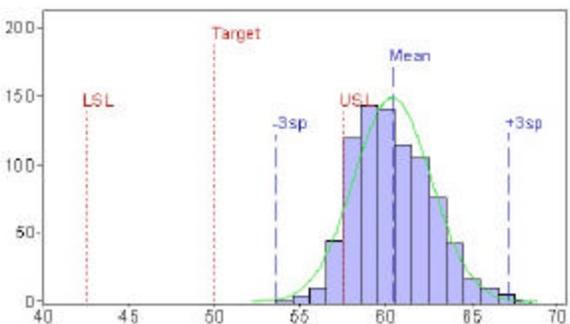
**Figure 10. 20 mil Resistor Data Compared to a target of 50 ohms - if no Attempt is Made to Scale the resistors, the Predicted Yield is Only about 10%**
