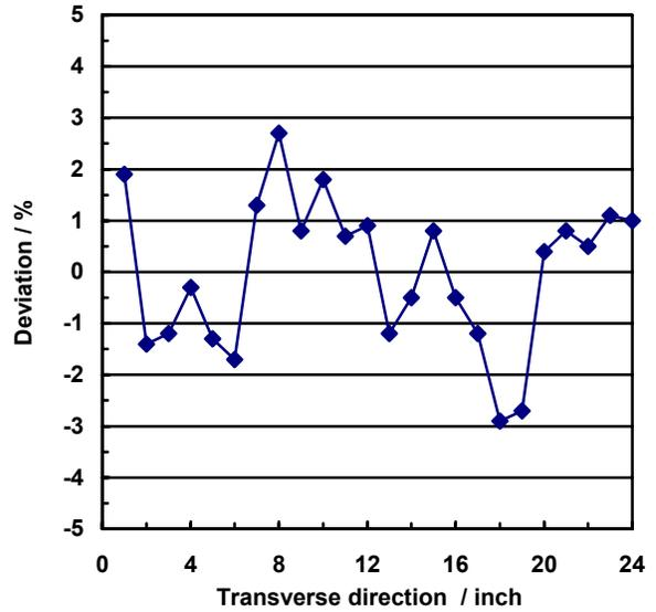
Figure 2: Sheet resistance uniformity in the transverse direction. Ni/Cr alloy on 1/2 oz RTC foil.
