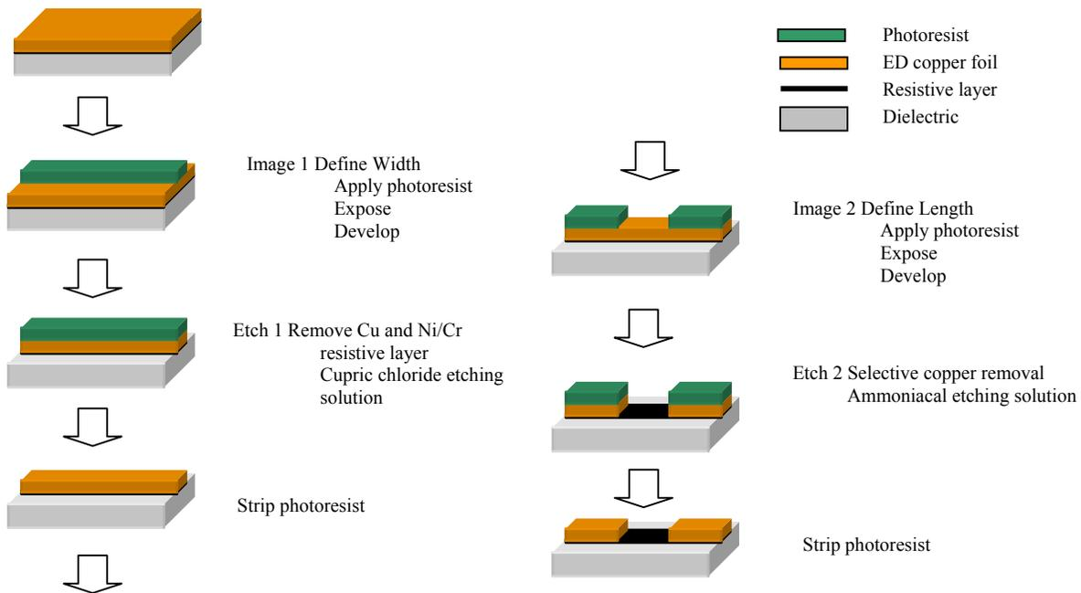
Figure 3: Schematic of etching sequence of Ni/Cr resistive layer.
