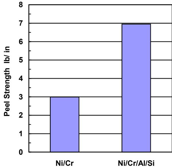
Figure 6: Peel strength of resistive material laminated on FR-4. Resistive materials sputtered on the untreated side of 12 $\mu$ m RTC foil. Sheet resistance is 100 ohm/sq.
