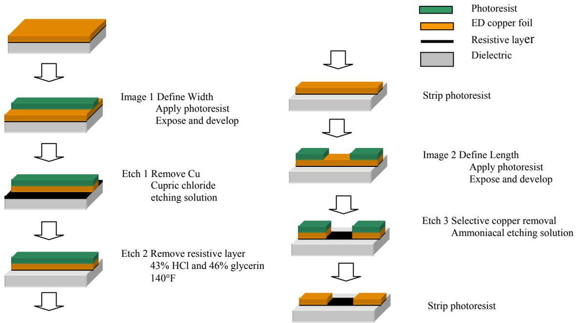
Figure 4: Schematic of etching sequence of Ni/Cr/Al/Si resistive layer.
