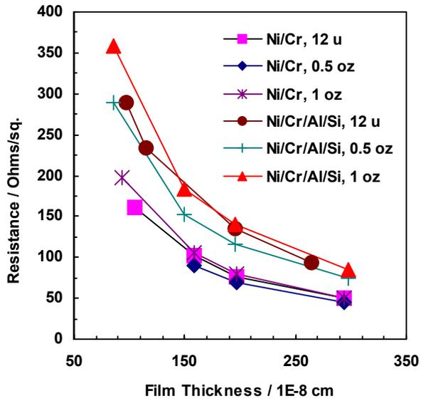
Figure 1: the correlation of sheet resistance to alloy film thickness and different copper substrates.
