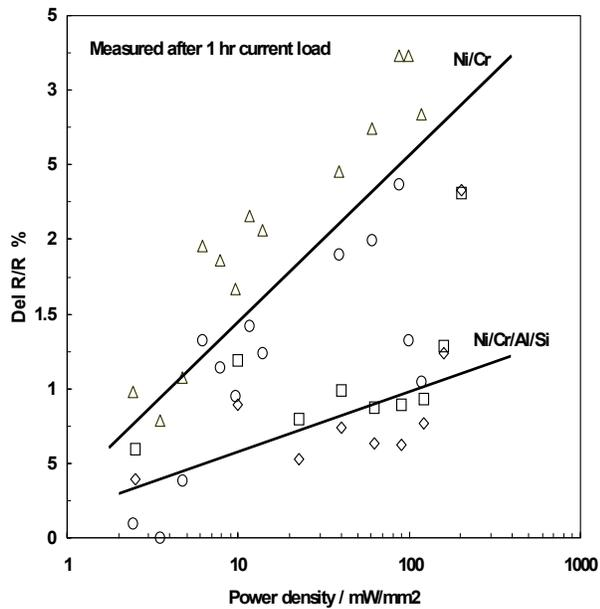
Figure 5: Resistance changes under current load. Resistive material was laminated on single side of FR-4 pre-pregs and the resistor size is 30 mil by 30 mil.
