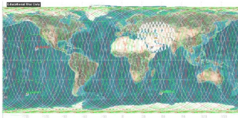
**Fig. 4 Track of sub-satellite point of co-planar orbit scheme**
