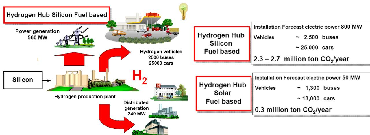
**Figure 2: Infrastructure of hydrogen production and distribution as well as the annual reduction in CO<sub>2</sub> emissions due to silicon based energy production.**
