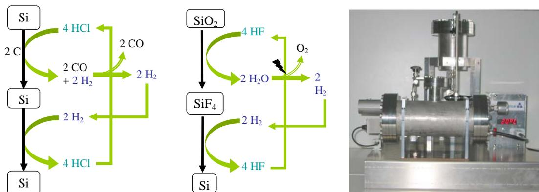
**Figure 1: Summary Chemical reactions for Production of Silicon from Sand. Prototype reactor for 1 kg H<sub>2</sub> is also shown**
