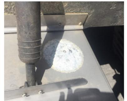
Alternatives to zinc anodes are available in aluminum and magnesium alloys, which have lower toxicity to marine life than the traditional zincs, as well as other potential performance advantages. Aluminum anodes work well in salt and brackish water, while magnesium are for fresh water boating. When switching to a different anode material, note that all the anodes on the boat must be the same material, and recommended to be a different metal than under-water components.
