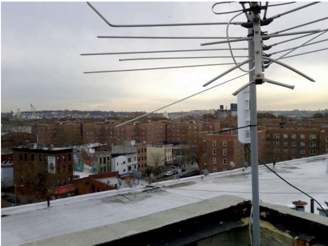
A Red Hook WiFi router serving Coffey Park, attached to an antenna | Photo by Jonathan Baldwin
