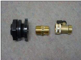
**A - Bottom Drain Installation:** Disassemble the bulkhead fitting. (Optional - Wrap Teflon tape around the long end of the brass hose adapter fitting) screw this into one of the bulkhead fittings. Once this is threaded into the fitting, thread on the brass shut off coupling until snug. This seals with a rubber gasket. Next, lay the barrel on its side, from the outside, insert the male end of the fitting through the 1½" hole at the bottom of the barrel, reach into the barrel
