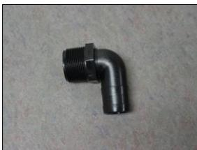
**C - Overflow Installation:** Thread in the overflow elbow into the 1½" hole near the top of the barrel. This is a tight fit, so it will require some elbow grease to get the threads started. You may need to use a file to open up the hole a little bit. Thread this all the way in, and stop when the barbed side of the elbow is pointing toward the ground, slip a five foot section of the sump drain kit hose onto the elbow.
