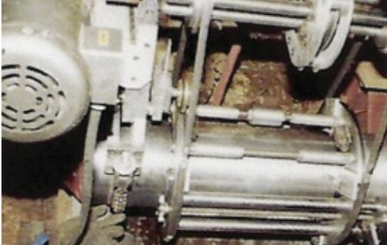
**STEP 1** - Pre-machining for weld overlay or sleeving of fan shaft
