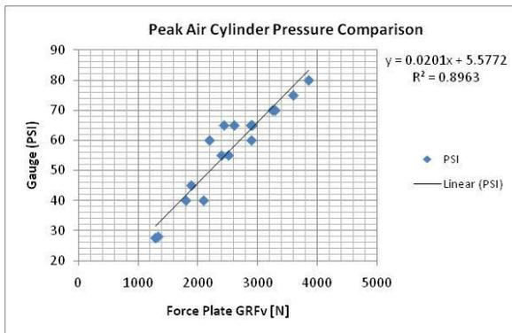
Figure 5: Comparison of peak PSI from pressure gauge and peak vertical platform ground reaction forces.
