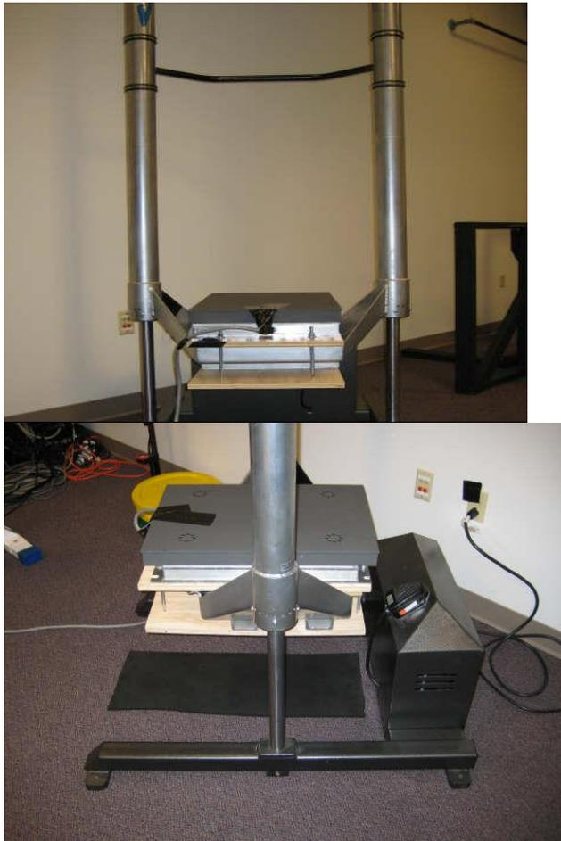
**Figure 1:** Front and side views of force platform mounted on top of Pneubounder foot platform.
