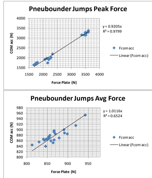
**Figure 2:** Comparison of peak (left) and average (right) vertical platform ground reaction forces on the Pneubounder using COM acceleration and the force platform, all jump styles combined.
