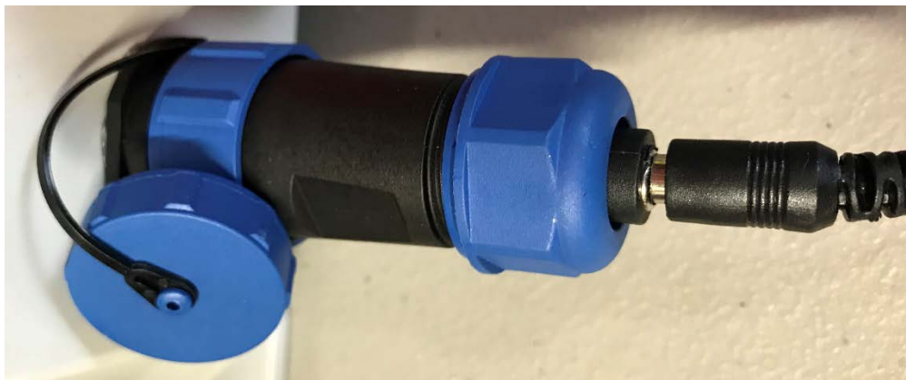
Figure 2.2a Thingy:AQ XC30 Connectors
