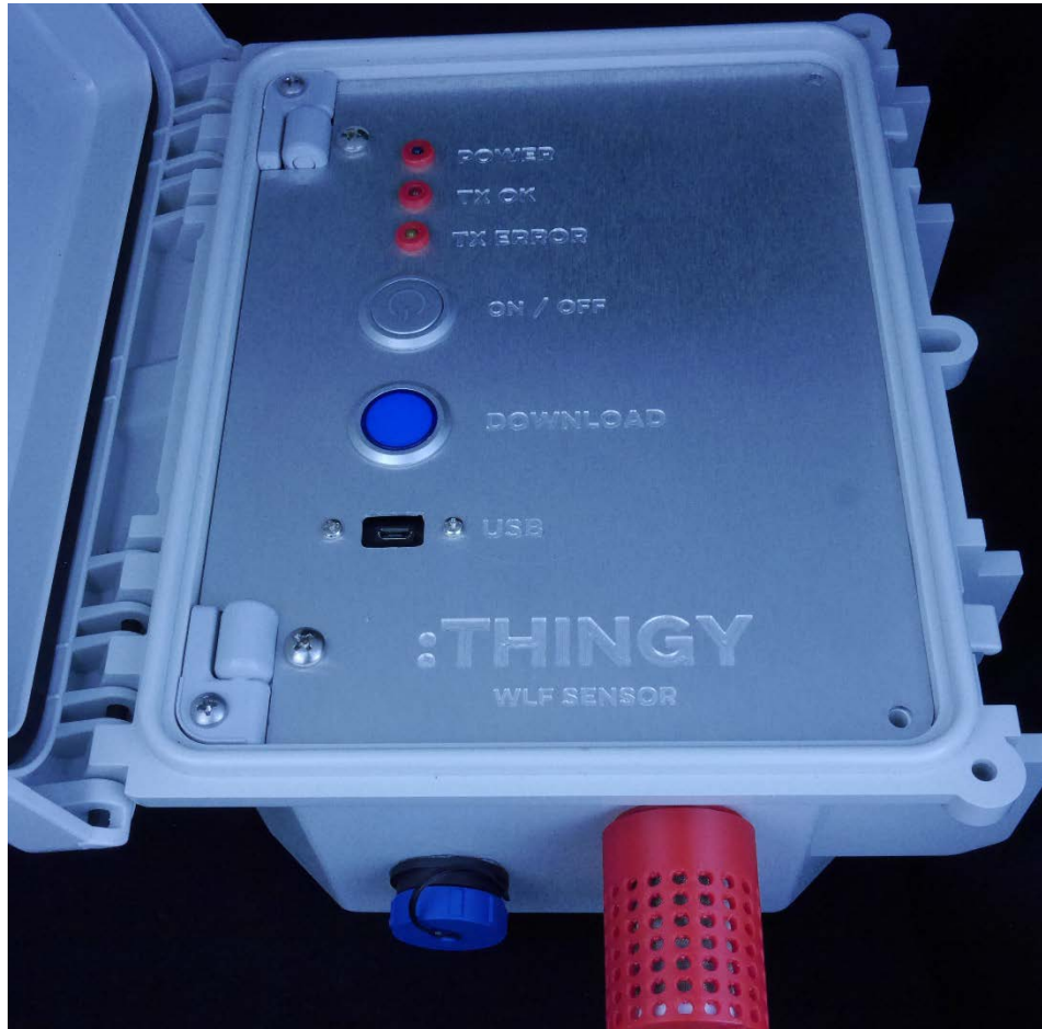
Figure 1.1 Thingy:AQ Sensor Node Housing with Inlet Air Filter
