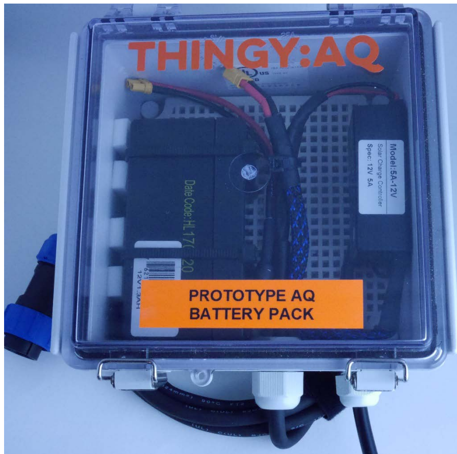
Figure 2.1 Thingy:AQ Sensor Node Battery Enclosure
