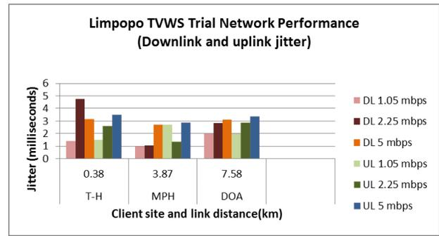
Figure 5. Downlink and uplink UDP jitter comparison results for selected links
