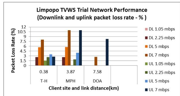
Figure 6. Downlink and uplink UDP packet loss rate comparison results for selected links
