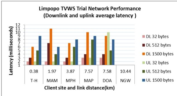
Figure 4. Average downlink and uplink latency comparison results per link
