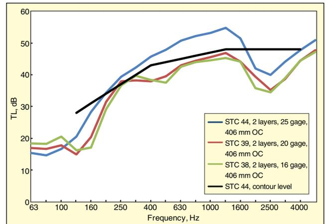
Figure 5. Transmission loss per frequency for a 1+1 layer partition with studs installed at 406 mm OC for various stud gages.
