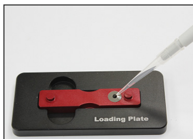
Pipette the Reference / Sample in turn.
