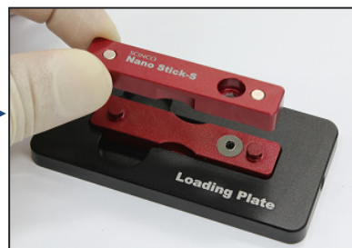
Assemble the upper plate to the other half.
