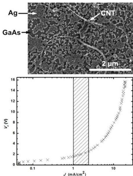
Fig. 4. (Top) SEM image of COOH-terminated CNTs deposited on 40-nm-thick sputter-coated Ag to clearly show Ag dissolution during negatively charged CNT deposition on positively biased working electrode. (Bottom)  $I$ - $V$  characteristic curve. Shaded region indicates the optimum operating range above which  $V_c$  rapidly rises with increasing  $J_c$ .
