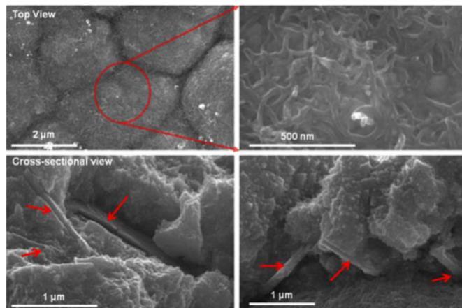
Fig. 5. (Top) SEM images of COOH-terminated CNTs deposited on electroplated Ag, using the nanospreader technique. Five successive layers of CNTs are deposited at a blade pull speed of 10 μm/s. (Bottom) Cross-sectional SEM images of Ag-CNT-Ag composite structure. The CNTs, indicated by red arrows, exhibit good adhesion to the surrounding Ag matrix.
