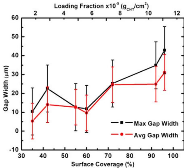
Fig. 10. Maximum and average gap widths achieved before lost connection as a function of CNT surface coverage and loading fraction.
