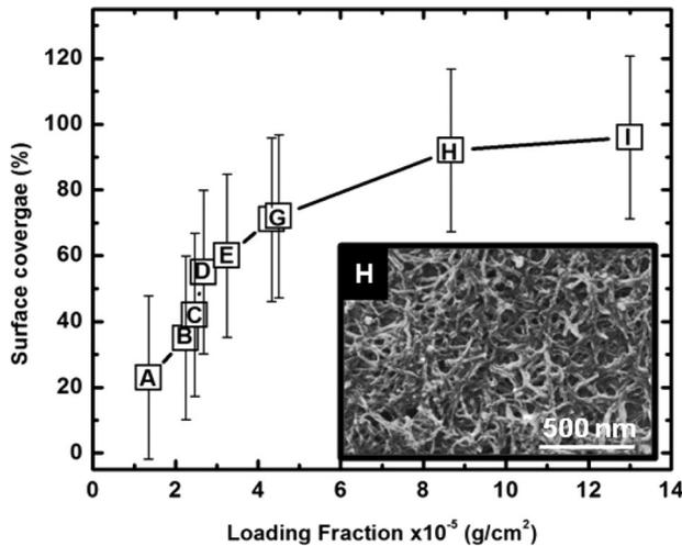
Fig. 7. CNTs loading fraction versus surface coverage with standard deviation bars. Past point H ( $> 9 \text{ g/cm}^2$ ), the surface coverage plateaus, asymptotically approaching 100%.
