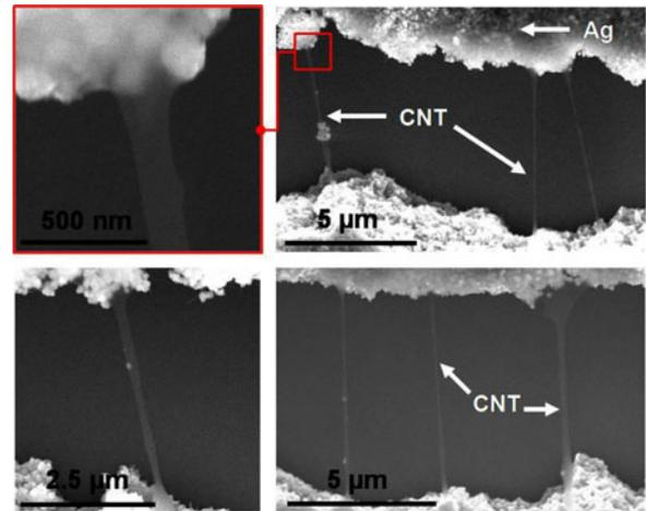
Fig. 11. SEM images of CNTs anchored in Ag layers clearly showing CNTs bridging cracks up to 9- $\mu\text{m}$  wide.
