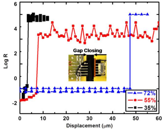
Fig. 8. Log plot of resistance versus gap across fractured MMC gridlines with three different CNT surface coverages. The connection is reestablished at 49, 9, and 5  $\mu\text{m}$  for samples with CNT surface coverage of 72%, 55%, and 35%, respectively.
