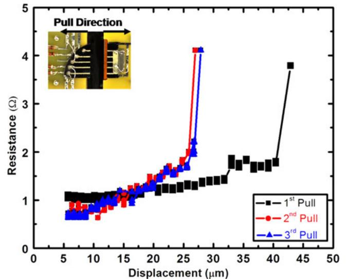
Fig. 9. Strain failure test of a MMC gridline (96% CNT surface coverage using drop cast method). The maximum gap at which the electrical connection is lost is reduced by  $\sim 34\%$  after the second pull test but remained constant after subsequent pull tests.
