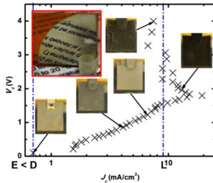
Fig. 2. Cathode potential  $V_c$  versus cathode current density  $J_c$ . The region between Point D and Point L defines the ideal operating window where the finish of plated Ag is bright.
