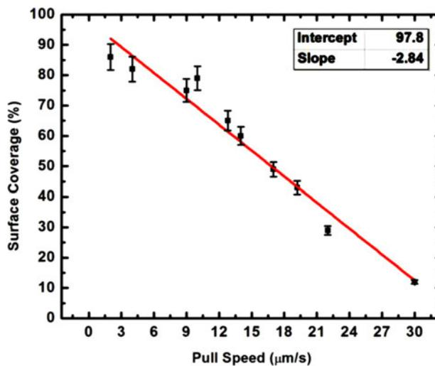
Fig. 6. Linear relation between the pull speed and corresponding surface coverage of CNTs using the nanospreader method.
