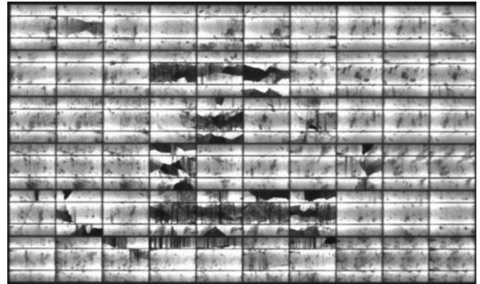
Fig. 1. Electroluminescence image of a microcracked photovoltaic module. Dark regions are electrically inactive areas [4].
