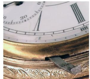
Setting a Lever Set watch is accomplished by gently unscrewing the front bezel (the ring that holds the crystal) remember righty-tighty, lefty-loosey. On hunter-cased pocket watches (those with a lid) the bezel does not
