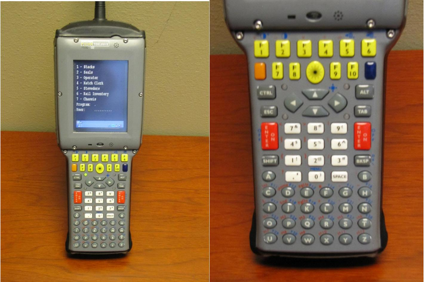
In addition to writing the location on your DISCHARGE SEQUENCE SHEET, you must INPUT the location. Start by pressing the red ENTER/ON button for a few seconds. If the handheld was completely off it will take a few minutes to connect to the base. When the blue screen comes up the cursor will be at the PROGRAM line. Press the white # 1 button for STACKS. Then push the grey down arrow V to the USER line and input the white #'s 7799. Hit enter and the STACKS screen on page 3 should appear.
