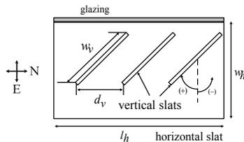
Fig. 2 Horizontal cross-section of shading devices.
