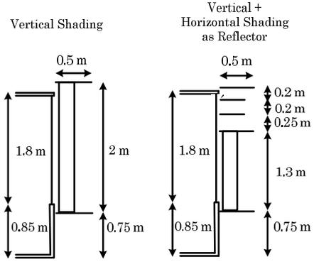
Fig. 3 Side-view of shading devices.
