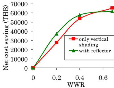
Fig. 7 Net Present Value of cost saving of two shading configurations due to WWR.
