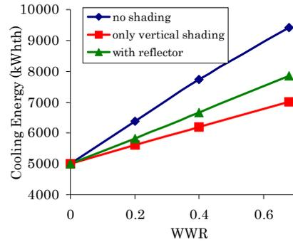
Fig. 5 Annual cooling energy consumption of external cooling load as function of WWR.
