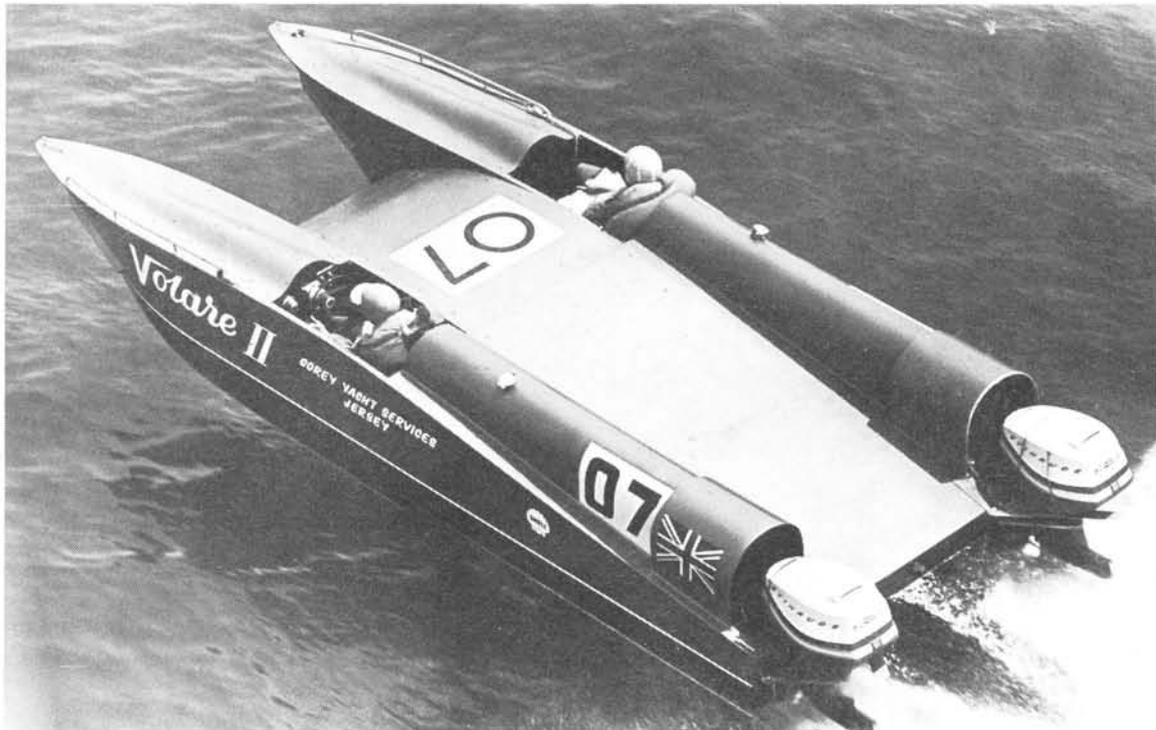
Third boat home, the comparatively tiny *Volare II*, driven by James Beard and Clive Curtis. Note the aerofoil centre section and the step halfway along the bottom of the hull.
