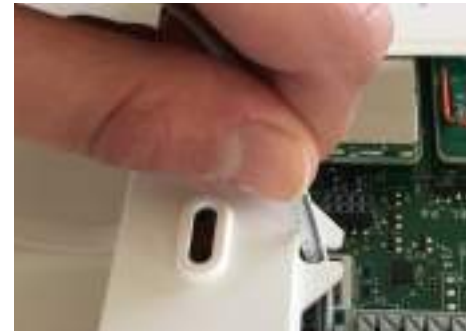
Insert the wire into the strain-relief
