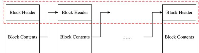
**Figure 1.** In the SVP scheme, a user stores the headers of the blocks, rather than the blocks themselves. A header contains the relevant meta data (e.g., the root of the Merkle tree whose leaves are the transactions contained in a block). This allows a user to verify whether a given block is valid or not.
