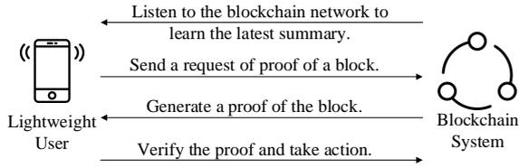
**Figure 2.** Illustration of the blockchain verification protocol. The nodes in the blockchain system with bigger storage capacities can keep a full copy of the blockchain. These nodes will interact with the lightweight users to help the latter to verify the validity of blocks.
