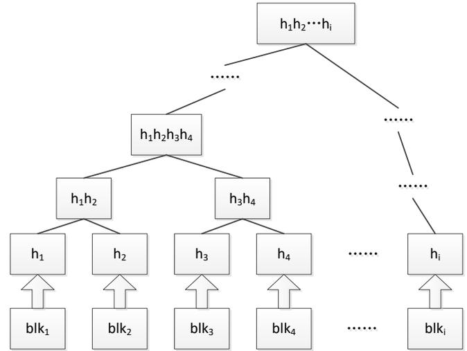
**Figure 3.** The storage structure that can be used by a prover to reduce its computational complexity when generating proofs. Each leaf  $h_i$  stores the hash value of a block, and each internal node stores the product of the values stored at its two children.
