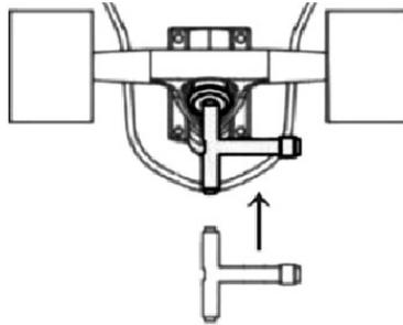
**Bushings:** The bushings are an indispensable and important part of skateboard, and users can adjust its tightness according to their weight and riding habits. Soft/loose bushings are easier for turning but it will make it unstable to ride at high speeds; hard/tight bushings are difficult for turning, but it will make it stable to ride at high speeds.
