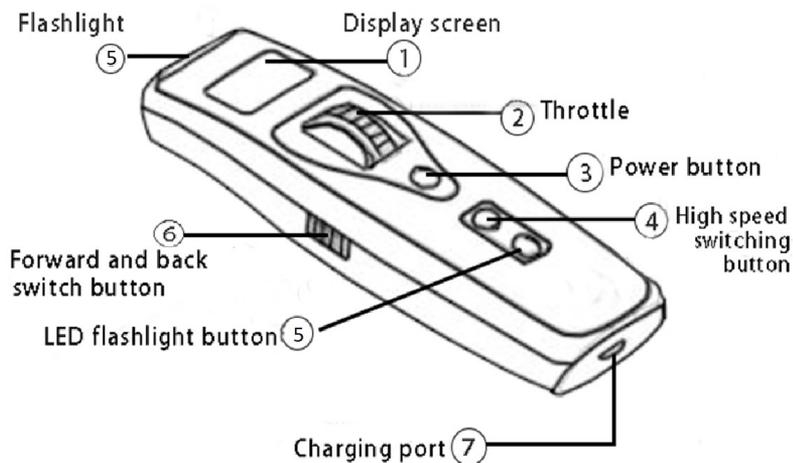
1) Display Screen: Real-time speed display, remote control and skateboard power display, remote control signal display, ODO skateboard cumulative and real-time mileage display, speed level, and braking level.
