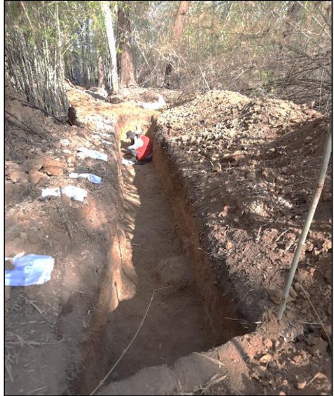
Near surface trenching to track the bends, pinches and swells of veins. Above: ANK staff sample veins every metre for assay. 19 samples submitted to ALS from this trench.
