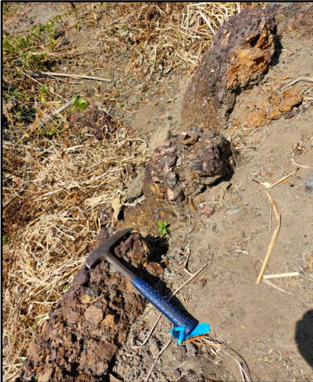
Exposed veins are collected by local landowner, who then crushes the material, and recovers 0 .41 gpt in gold.
