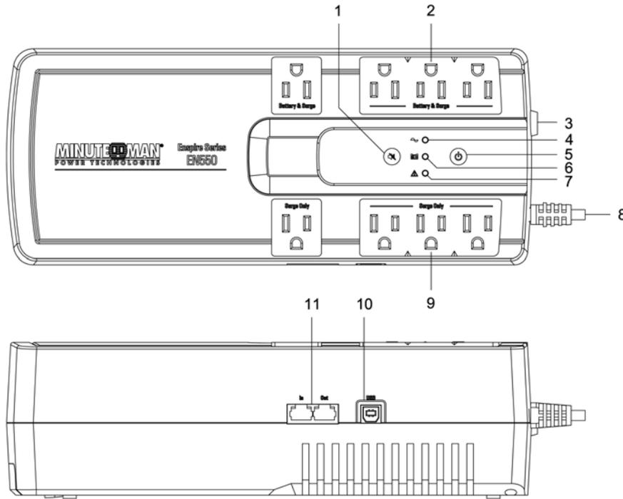
1. Alarm Silencer Button: Silences the alarm during the Battery mode.
