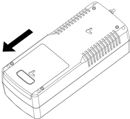
7. Lift the battery door upwards, remove the battery module by pulling the pull-tab, and then set aside. (FIG. 2)
