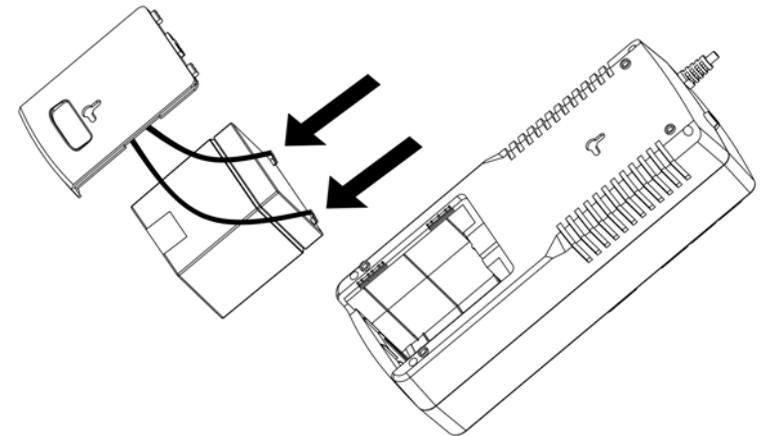
12. Slide the new battery module into the UPS.
