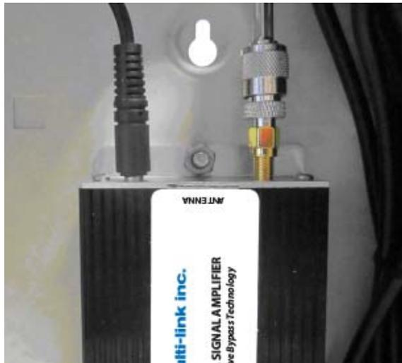
9. a) For installation in a commercial UL 1610 application – Connect the hardwire power cable to a listed compatible UL 1610 Panel, Dialer or Power Supply listed for Fire with limited power regulated outputs.
