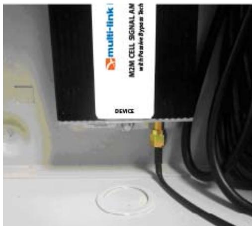
7. Connect the SMA-to-SMA device cable to "Listed Compatible" cellular device.
