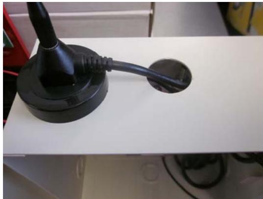
4. Connect the SMA end of the Antenna cable to the ML-CSA 3550 UL connection marked "Antenna".
