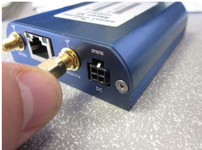
**B) Connect the MMCX end of the SMA to MMCX device cable to the Cellular Module.**
