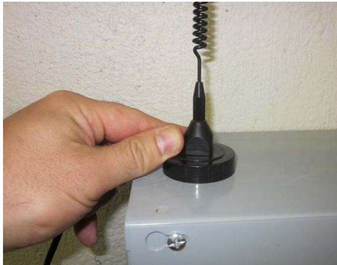
**B) Mobile - Mount the Outdoor Signal Antenna (#4 on Parts List) vertically on any metal surface on the roof, hood or trunk of the vehicle.**
