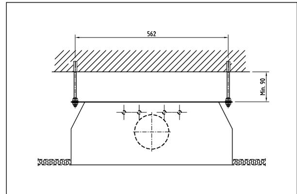
Figure 7. Polaris I 60 recessed in a suspended ceiling.
