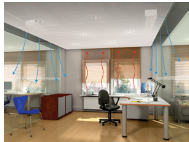
Picture 2. Celo's technical solution is based on a unique technology, patent applied for, where the cooled air is carried down through an outlet slit in the suspended ceiling, then along the wall and down towards the floor.
