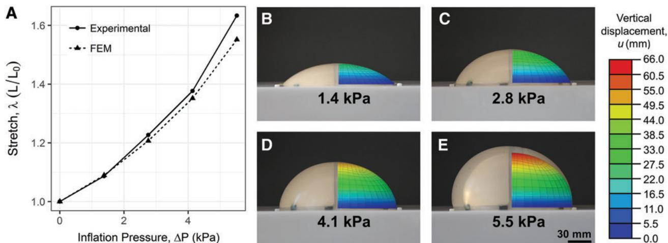
**FIG. 5.** Stretch of the elastomeric membrane during inflation. (A) Aggregate stretch across the profile of the HLEC membrane as internal pressure is applied. Experimental results are compared with results of a numerical simulation. Profiles of the device are shown alongside vertical displacement,  $u$ , for pressures of 1.4 kPa (B), 2.8 kPa (C), 4.1 kPa (D), and 5.5 kPa (E). Color images are available online.
