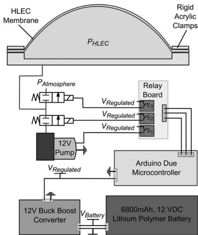
**FIG. 4.** Pneumatic control system for the untethered HLEC interface. A pair of two-way, normally closed directional valves are used to alternate between inflation by using a 12 VDC pump, holding pressure, and venting to the atmosphere.
