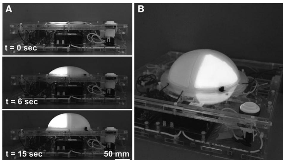
**FIG. 1.** Four HLECs form an untethered soft interface that is capable of emitting light and sensing touch. (A) The membrane is pressurized by using an integrated pump. (B) Fully inflated HLEC interface with one panel illuminated by using applied voltage,  $V \sim 4$  kV, and frequency,  $f \sim 1$  kHz. HLEC, hyperelastic light-emitting capacitor.
