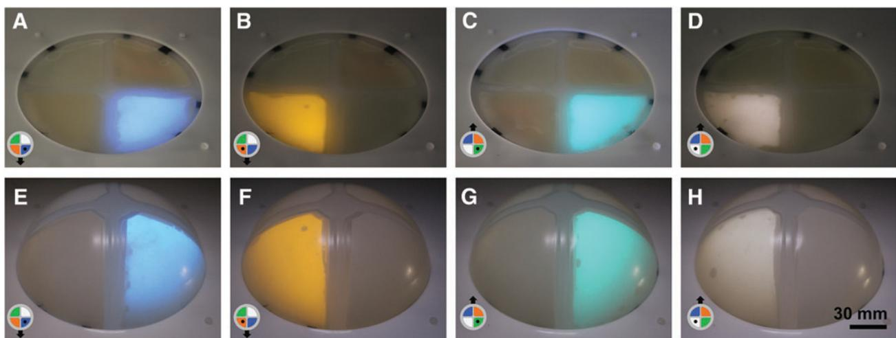
**FIG. 8.** Illumination of the HLEC panels. *Blue* (A), *orange* (B), *green* (C), and *white* (D) panels are illuminated whereas the membrane is uninflated. *Blue* (E), *orange* (F), *green* (G), and *white* (H) panels are illuminated whereas the membrane is pressurized to  $\sim 4.1$  kPa. Color images are available online.
