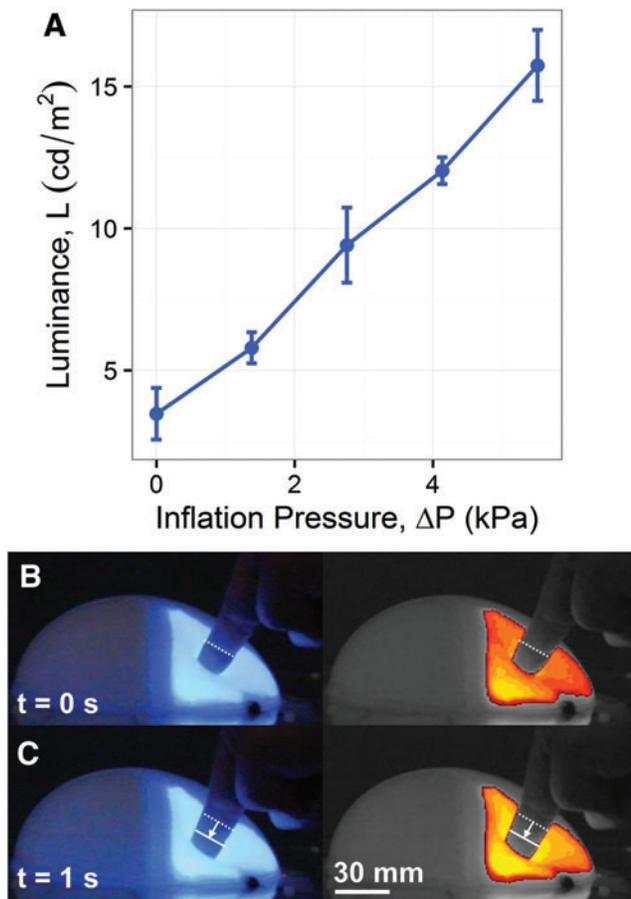
**FIG. 7.** Change in luminance during deformation. (A) Luminance for the *blue panel* as the membrane is pressurized. Error bars represent the standard error calculated by using three measurements. (B, C) Pressurized HLEC panel being deformed with a finger press while illuminated. The images on the *right* show the relative luminance of the device, with *yellow* coloration corresponding to the highest luminance. Color images are available online.
