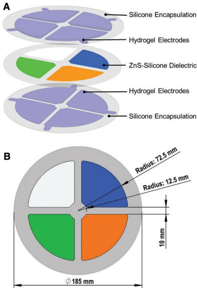
**FIG. 2.** Design of the elastomeric membrane with four independently controlled HLEC panels. **(A)** Exploded view of the membrane showing its five-layer structure. A 1-mm-thick electroluminescent dielectric layer is sandwiched between hydrogel electrodes, and the device is encapsulated with a final layer of silicone. **(B)** Dimensioned drawing of the dielectric layer. The active area of the device has a 145-mm diameter, with a 20-mm border for mounting. Color images are available online.
