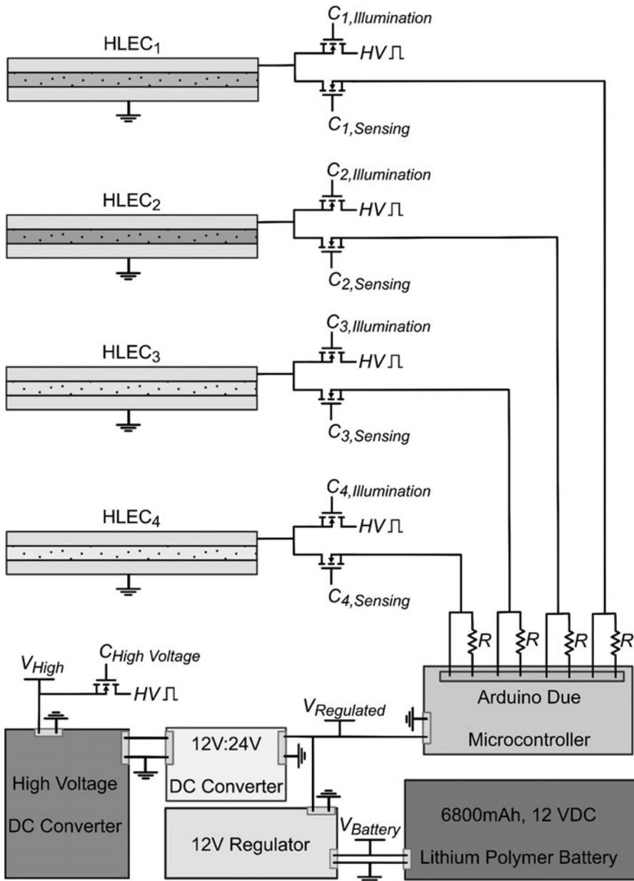
**FIG. 3.** Electronic design for untethered illumination and touch sensing. One electrode from each HLEC is grounded, whereas the other is switched between a high-voltage square wave for illumination and a low-voltage signal for capacitive touch sensing.
