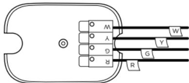
4. Open up the PEK. It has two rows of terminals (one side is for thermostat connections, the other side, pre-wired, is for the control board connections).
