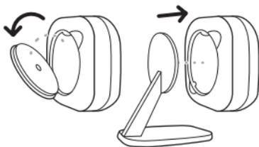
..... To remove the remote sensor stand, pull the base outwards.
