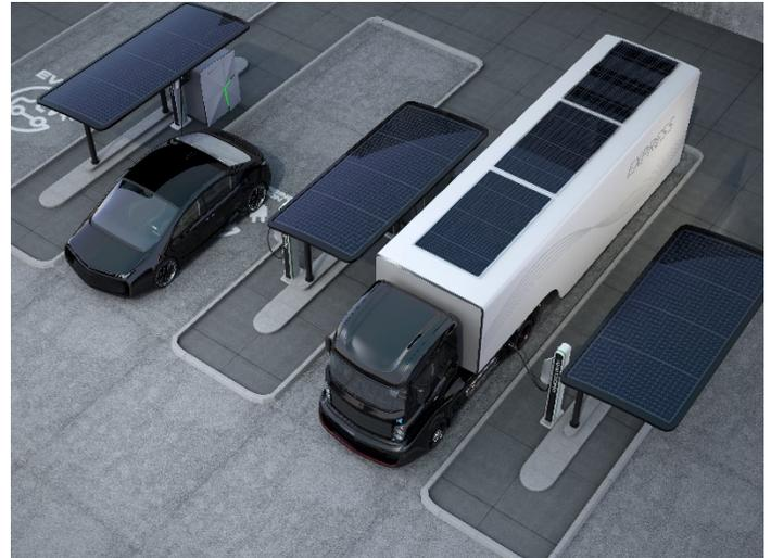
the average passenger EV only utilizes roughly 10kWh of power per day, while an electric school bus uses 6 to 12 times that amount (between 60kWh and 120kWh of energy per day) Public transit buses and other heavy vehicles can use over 400kWh of energy per day.
