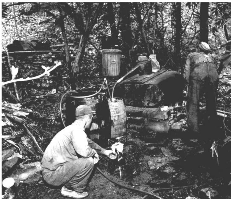
Figure 2. Two unidentified men operate a submarine-style moonshine still, Franklin County, Virginia, 1950s. By mid-century, most moonshiners had learned that stills made with galvanized sheet metal were far more efficient than ones made with rock and mud. Credit: "Moonshining photo #78," Earl Palmer Collection, Blue Ridge Institute and Museum at Ferrum College.
