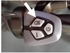
To turn on the Backlight, press the Light Button on the Thumb Pad.
