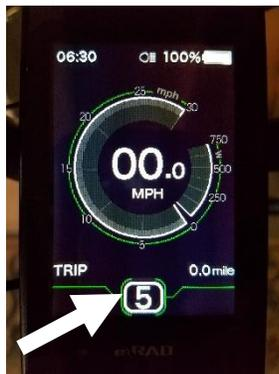
The throttle provides full power in all power assist levels including 0 but, for safety reasons, the throttle will not work until you start pedaling. When using pedal assist, the power will begin when you begin pedaling.
