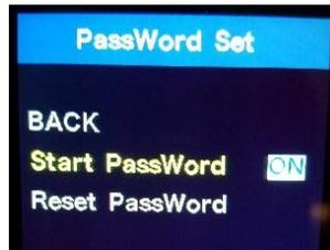
Press Mode. Press + or - to select ON. Press Mode. Press + or - to switch between numbers. Press Mode to lock in number and move to next number.
