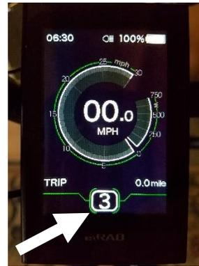
The + and - buttons on the left side of the thumb pad access different levels of pedal assist; 1 being the lowest assist level and 5 being the highest.
