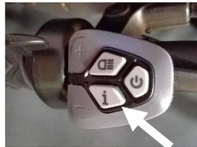
To access the Display Setting screen to the right, press the Mode Button quickly 2 times. Display Setting will be highlighted. Press Mode again to get to the Display screen shown.
