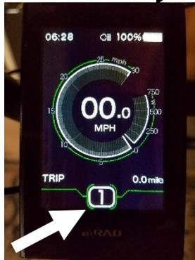
Hold Power Button for two seconds to shut system down.
