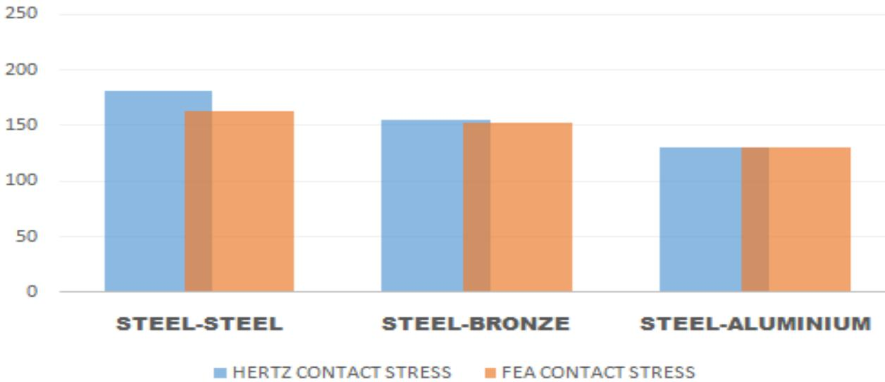
Fig. 4.1 Graph showing the comparison of contact stress values obtained from Hertz equation and FEA Analysis (Values in Y-axis represents contact stress in MPa).
