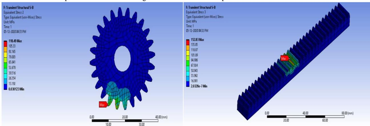
Fig. 4.4 Contact stress on pinion (Steel-Bronze combination); Fig. 4.5 Contact stress on rack (Steel-Bronze combination)
