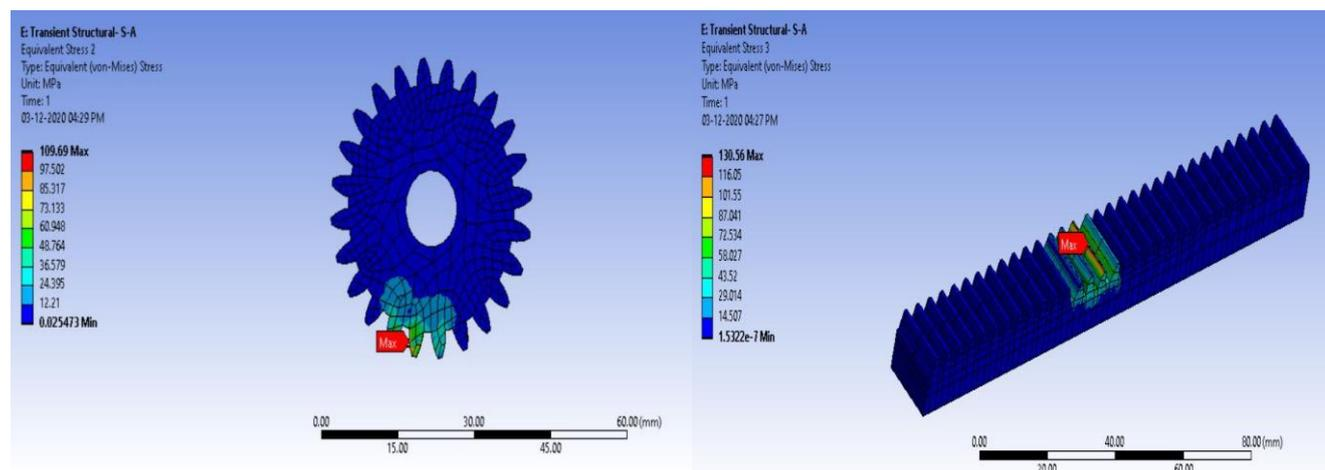
Fig. 4.6 Contact stress on pinion (Steel- Aluminium combination); Fig. 4.7 Contact stress on rack (Steel-Aluminium combination)
