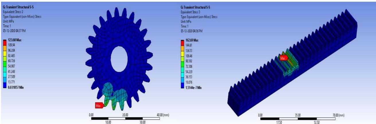
Fig. 4.2 Contact stress on pinion (Steel-Steel combination); Fig. 4.3 Contact stress on rack (Steel-Steel combination)
