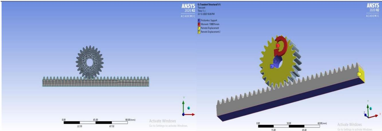
Fig. 3.3. Finite element model of Rack and Pinion; Fig. 3.4. Constrains on Rack and Pinion
