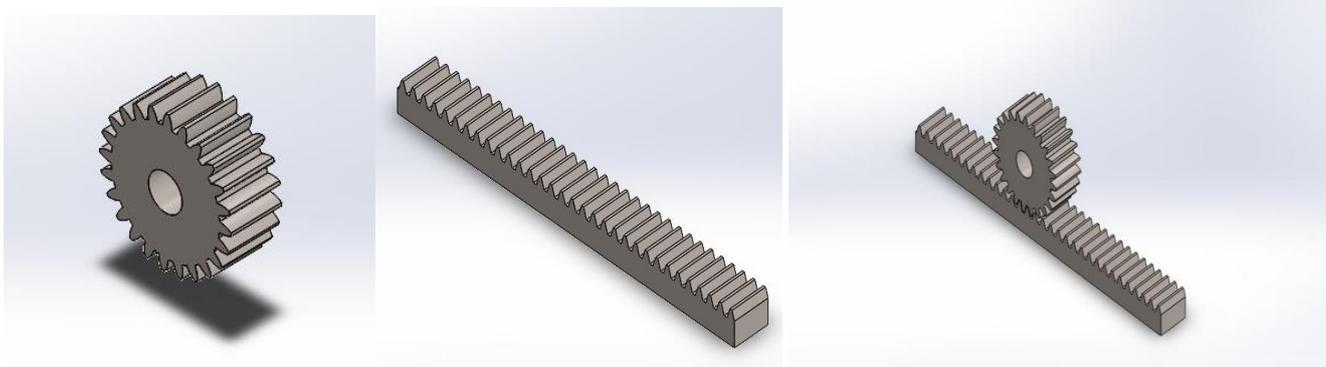
Fig.3.1. CAD model of Rack and Pinion; Fig. 3.2. Meshed assembly of Rack and Pinion
