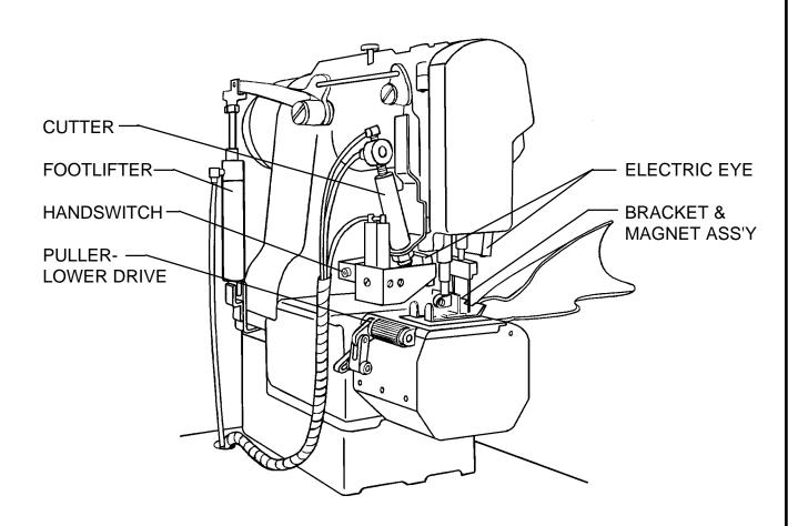
The Clinton Model 315NA-TA600 is an impact thread cutting and waist band puller system especially designed for the Seiko DC-27 Bander. An LCD programmable controller is used with electric eyes to sense the leading and trailing edge of the garment and control foot lifter, cutter, puller, limit speed and maximum speed sewing.
