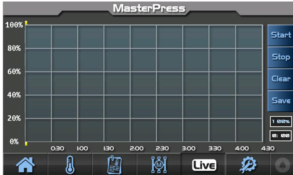
1. Press anywhere in the graph area a dot will appear this is the GO TO point , build a profile in this page then press START and it will run the on screen data points. Pause will appear in the run mode to pause the action.
