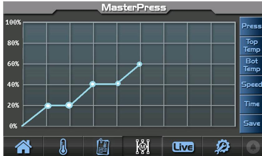
1. This shows the PROFILE , time is on the bottom and pressure is on the side , it is a RAMP/SOAK profile , it will ramp over time to the next position these are the ramps.
