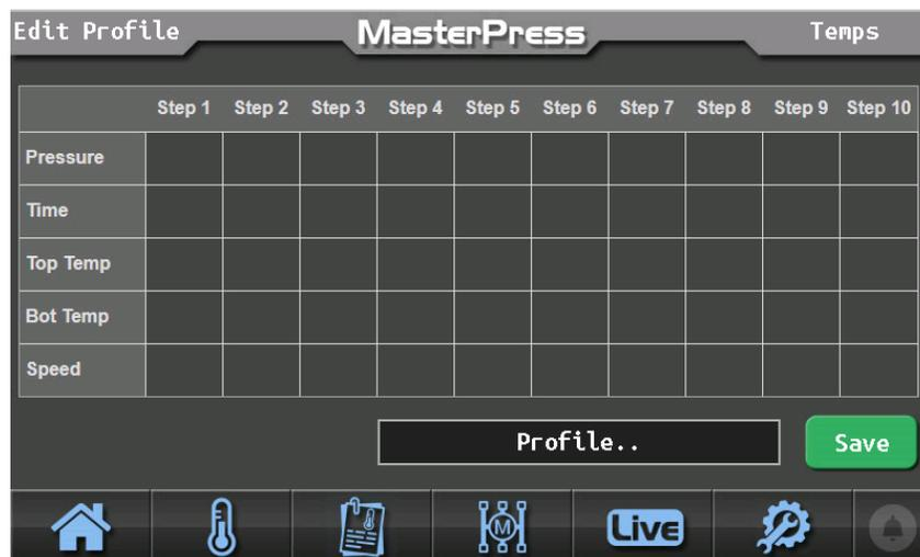
4. Copy is to copy a profile to a new memory spot. Select the profile you want to copy then press copy, scroll to the profile you want to store that copy in and press paste. You can then edit the profile and rename it.
