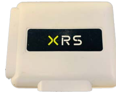
XRS Relay (Connected to Vehicle ECM)
