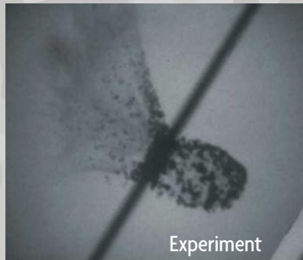
Both experiments were modeled with the  $\gamma$ SPH™ Solver using a linear elastic-plastic constitutive model and Mie-Gruneisen equations of state. The correlations with the experiments are excellent showing the accuracy of the  $\gamma$ SPH™ Solver. This figure shows very good comparison of the resulting debris cloud.
