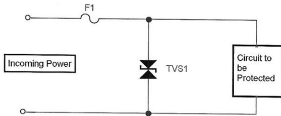
If however the fuse is placed in this manner the fuse opening will not affect but will disconnect the load.
