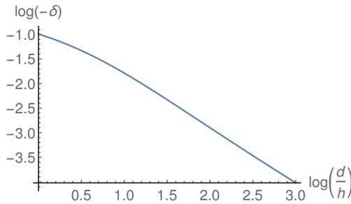
FIG. 9. Logarithm of the fractional reduction in the vicinity of the right upper corner of the emitter showed in Fig. 1 as a function of the logarithm of the ratio  $d/h$  for  $\xi(x, y) = \eta(x, y) = 0.0001$ .
