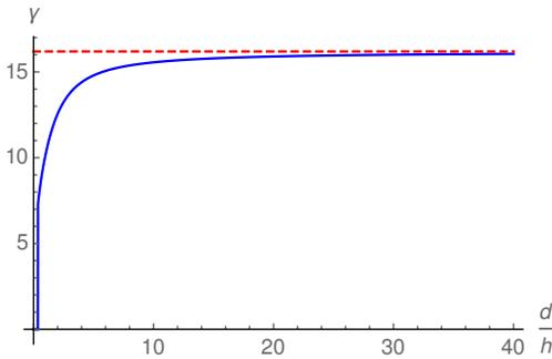
FIG. 5. FEF in the vicinity of the right upper corner of the emitter in Fig. 1 for  $\xi(x, y) = 0.0001$ . The (red) dashed line corresponds to the same FEF ( $\eta(x, y) = 0.0001$ ) in the case of a single emitter showed in Fig. 3.
