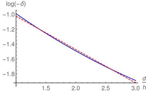
FIG. 8. The (blue) filled line represents a restriction of the plot in Fig. 7 for small values of  $d/h$ . The (red) dashed line shows a linearization obtained from using 20 equidistant points from the plot in Fig. 7.
