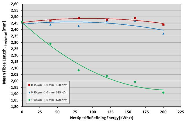
Figure 5: At the same bar width of 1 mm, large length reduction takes place between 335 and 670 N/m.
