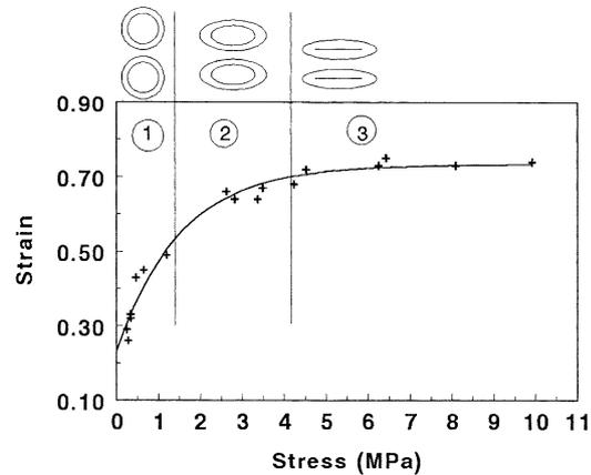
Figure 3: Fibre compression (from Amiri and Hoffmann 2003).
