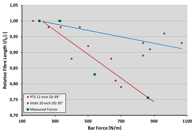
**Figure 7:** Data from Studies A and B for refining energy 160 kWh/t show an envelope of fibre shortening and bar force. Data measured by a force sensor fall near the Study A line.
