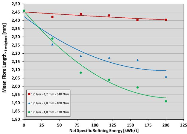
Figure 4: At same SEL = 1 J/m, bar forces over 300 N/m gives large fibre length reduction.
