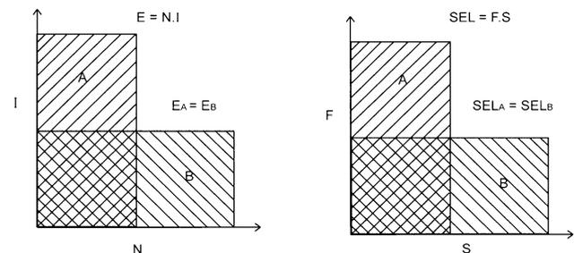
**Figure 2:** Illustration of Specific Edge Load (*SEL*) as the product of bar force and sliding distance over which force is exerted, analogous to energy factored into number and intensity of impacts (Kerekes 2015).
