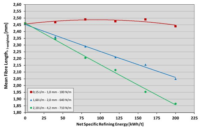
Figure 6: For bar widths 4.2, 2.0, 1.0 mm and SEL's 2.1, 1.6, 0.3 J/m, large length reduction occurs between bar forces 100 and 640 N/m.
