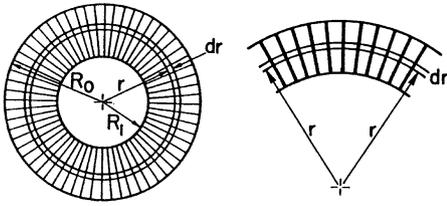
Figure 1A: Schematic of refiner plate.
