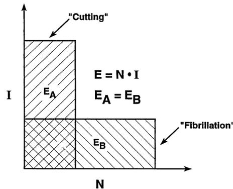
**Figure 1:** Illustration of Specific Refining Energy as the product of number and intensity of impacts on pulp (Kerekes 1990).
