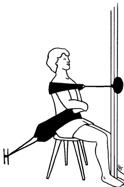
**Fig 7.** Drawing shows Darcus strain-gauge dynamometer. Subject sits on stool facing testing apparatus, vertical bar is fixed to axis of dynamometer, and subject is attached to bar with strap around shoulders. Strap around hips prevents forward movement of pelvis.
