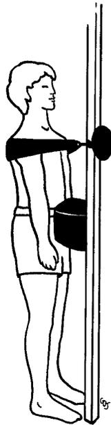
Fig 5. Drawing shows pulling test described by Jorgensen and Nicolaisen.<sup>9</sup> Subject stands facing strain-gauge dynamometer, is then strapped to dynamometer, and attempts maximal backward extension while pelvis is supported. Subject pulls at 60% of MVC under control of supervisor until no longer able to maintain 60% value.
