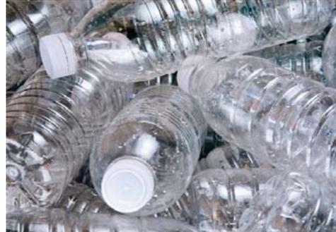
2. The discarded soda and drinking bottles are cleaned and cut into flakes before being melted and extruded into fibres of natural white colour.
