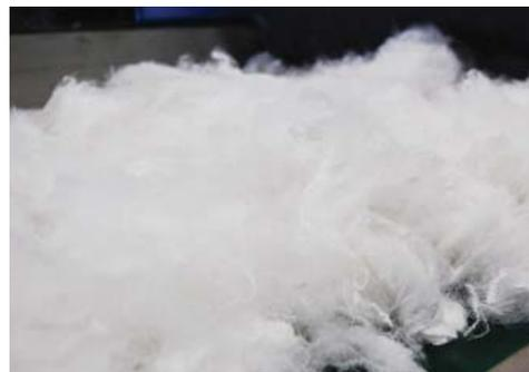
4. The regenerated fibres are then integrated into the carded multi layerweb construction and thermo bonding process to create new material for acoustic panels.
