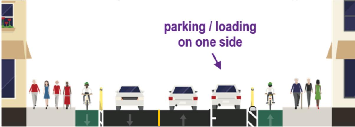
Example of proposed street configuration for narrow sections: bike lane with on-street parking on one side
