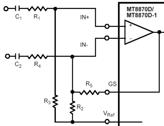
**Fig 3 The figure shows the differential configuration, which permits the adjustment of gain with the feedback resistor R5.**
