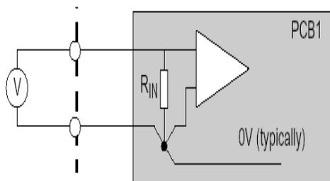
Fig 4 Diagrammatic representation of grounding technique.
