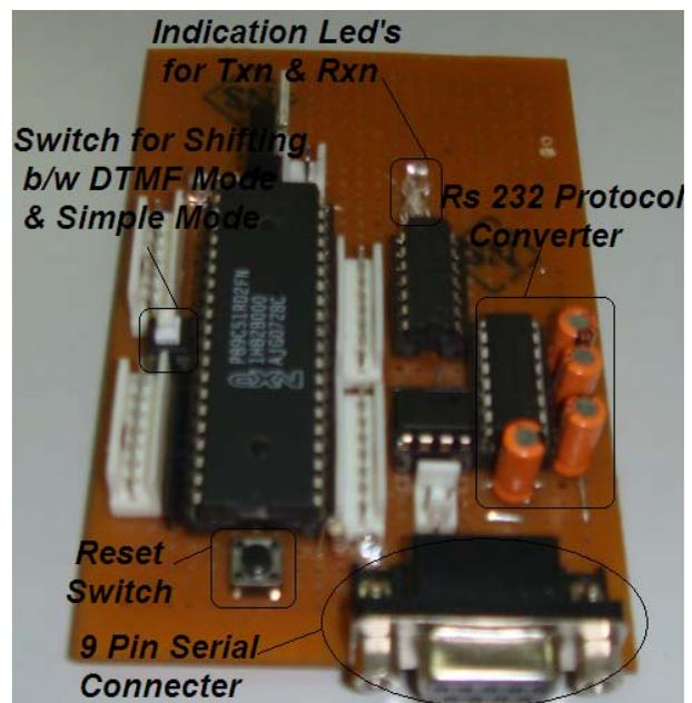
Fig 5 A In-System Programmer Circuit
