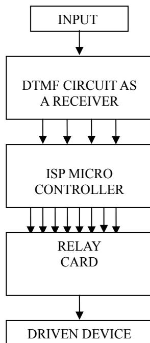
**Fig 1 Functional block diagram**
