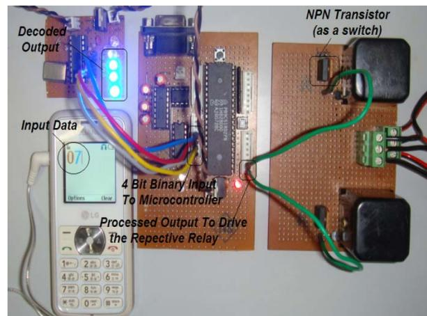
**Fig 8 The Complete Interfaced System**
