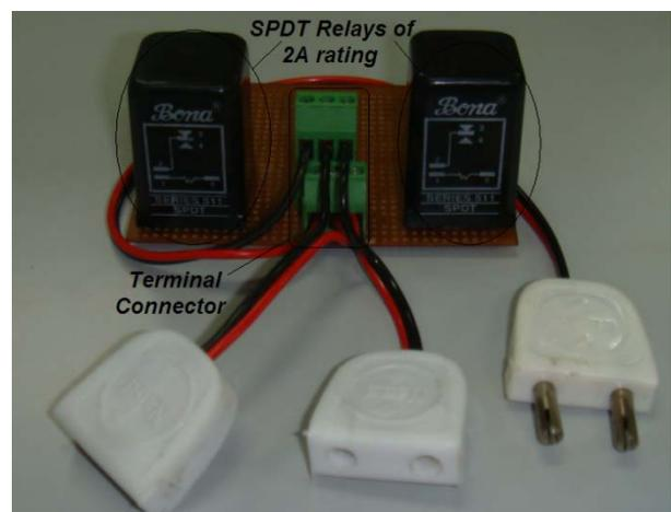
**Fig 6 A two relay, Relay Card used to drive a device**
