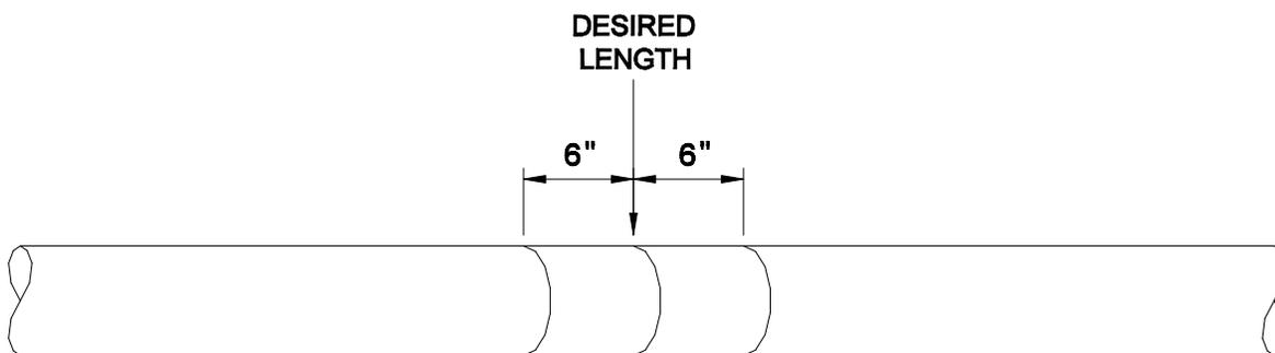
Use a carpenter handsaw or PVC saw to cut the PVC or HDPE casing. Be careful not to damage the FRP carrier pipe during this cutting operation. Remove the casing and cut off the insulation. See illustration below.
