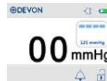
**Mode: Continuous mode:** The solid line indicates Continuous mode. In Continuous mode, the device will always maintain the set pressure.
