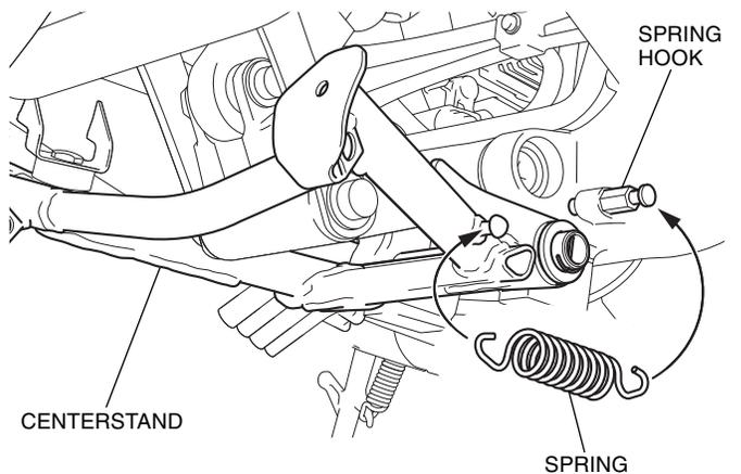
14. Install the motorcycle's parts in the reverse order of removal.
