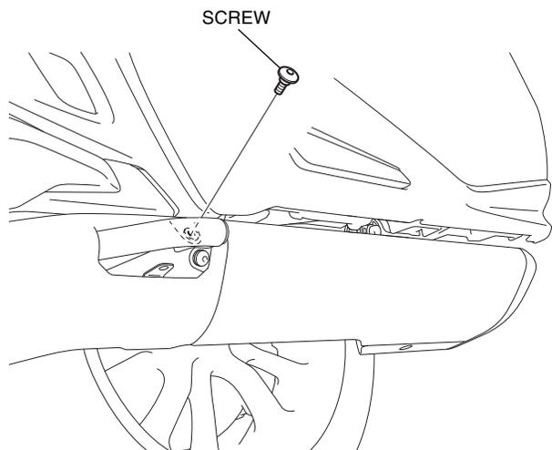
3. Remove the left exhaust pipe cover as shown.
