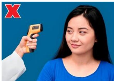
Figure 2: Incorrect Use – Not perpendicular to the forehead
